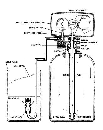
Hard water enters the unit at the valve inlet - flows around the lower piston groove - thru the injector throat - thru the brine valve and flow control to fill the brine tank. Hard water also flows around the lower piston groove - thru the passage to the top of tank - down thru the resin and enters the distributor as conditioned water. The conditioned water flows up thru the center tube to the valve outlet.
