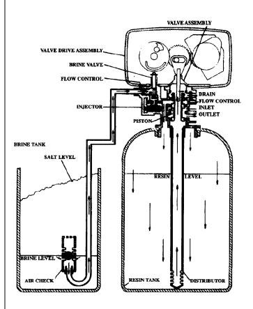
Hard water enters the unit at the valve inlet - flows around the lower piston groove and lower piston land - down thru the center tube and out the distributor - up thru the resin - thru the top of tank passage - around the upper piston groove and out the drain line.
