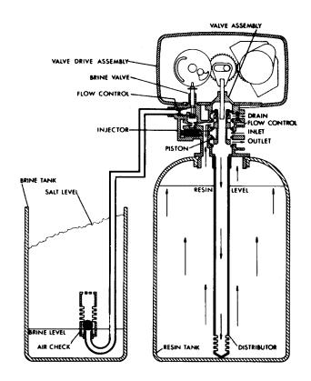
After all the brine has been drawn from the brine tank, hard water continues to enter thru the valve inlet - flows around the lower piston groove - thru the nozzle and orifice - down thru the resin and into the distributor - up thru the center tube - thru the center hole in the piston and out the drain line.
