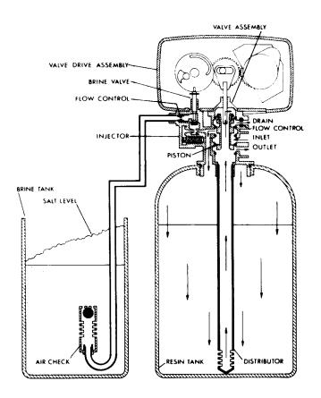
Hard water enters the unit at the valve inlet - flows around the lower piston groove - thru the passage to the top of tank - down thru the resin and enters the distributor as conditioned water. The conditioned water flows up thru the center tube to the valve outlet.
