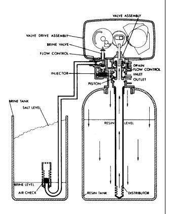
Hard water enters the unit at the valve inlet - flows around the lower piston groove - down thru the top of tank passage - downward thru the resin - up the distributor tube - thru the center hole in the piston - over the top edge of the piston and out the drain line.
