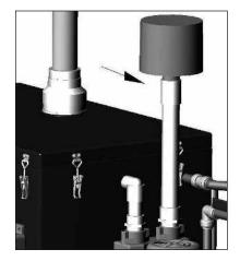
**Figure 10** Air Intake Connection
