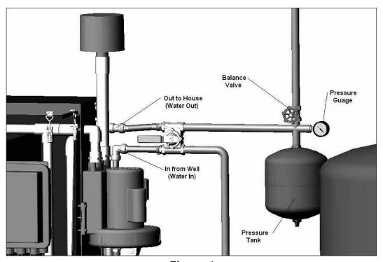
**Figure 4** Water Connections
