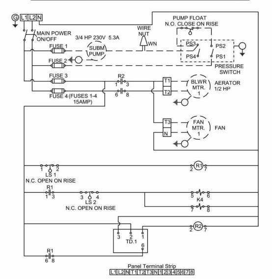
Black White Red Component Green Power In (230V) L1 N L2 Ground On/Off Float (middle) 2 1 Fail Safe Float (upper) 3 4 5 6 Solenoid Ground 7 Solenoid 8 Ground Blower T1 T2 Ground Pump Fuse 1 WN Ground Vent Fan (if used) N Ground T3 Pump Float (lower) PS3 PS2 WN-PS3 FUSE 2-PS1 Pressure Switch Ground
