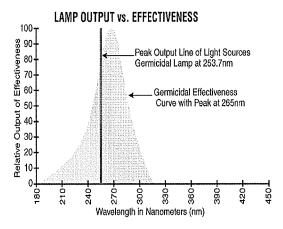
Standard low-pressure lamps produce close to 95% of its light in the 254-nanometer range. The sensor head contains a quartz-filtering device that blocks all wavelengths except those required for the destruction of microorganisms.
