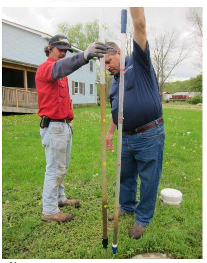
Comparison of solids settling in tanks in a NY site:
