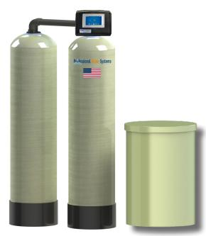
Hard water passes through the online media tank that contains resin beads coated with sodium ions. The calcium and magnesium ions are exchanged for sodium (or potassium) ions, thus softening the water. When the beads have trapped the hardness and need to be regenerated, the Pro H20 control valve charges them with the brine from the brine tank.
